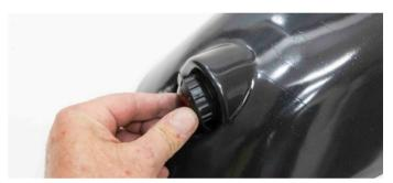
Inside the installation package, you will find a special drill that will help you drill a hole for the tail light. Following this, push the tail light in the hole until it fits.
